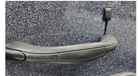
Gunnel mounted switch - wire hidden behind grab handle
